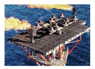
Darscreen<sup>TM</sup> - radiant heatshield system can be used as a horizontal heatshield directly below the flare tip, but is commonly used for vertical heatshield protecting critical plant equipment, steelwork and personnel.
