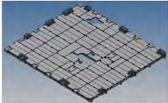
Darflare™ heat shield model – overall design showing panel arrangement, access points and hand rail & pulling posts
